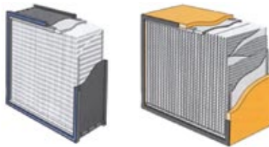
Esco cabinets use Swedish Camfil Farr® mini-pleat filters without aluminum separators to increase filter efficiency, minimize the chance of leakage, and to prolong filter life. Filters include a lightweight aluminum frame for structural stability and elimination of swelling common to conventional wood frames.
