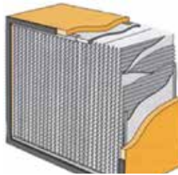
Fig 4. Pack is glued into a frame - Frame is gasketed to form final assembly
