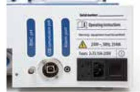
BNC connection for pH monitoring, USB communication port, and port for external alarm monitoring
