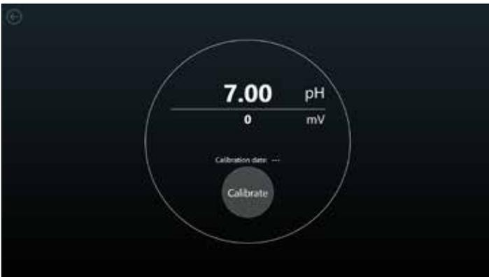
The Miri® TL has a built-in standard pH meter (BNC-type connection pH probes) and is accessed from the pH meter screen.
