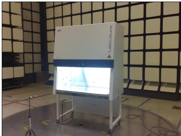
The cabinet voltage and inflow velocity was first verified prior to testing, to ensure that it operates on same factory setting. Inflow measurement was performed on-site using Airflow AV30 anemometer, which confirms the inflow of 0.45 m/s, which is the normal operating point of this cabinet.
