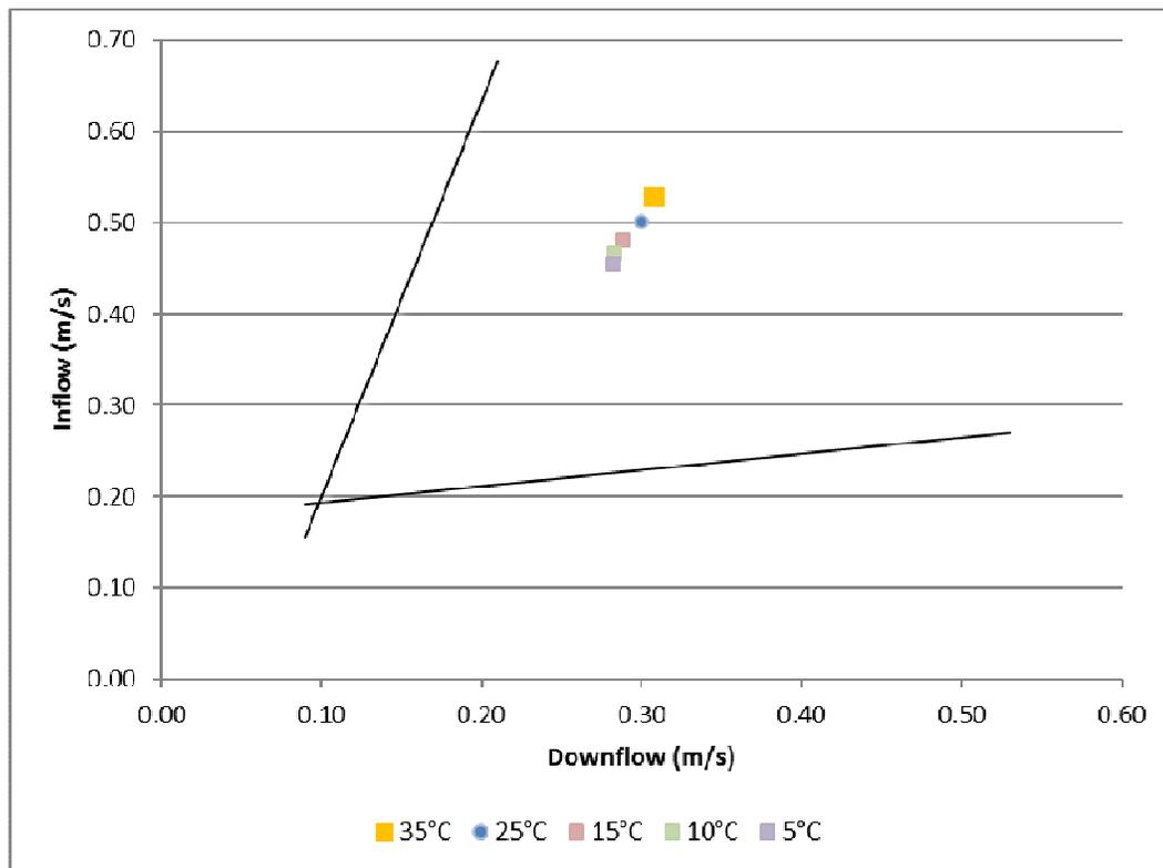
Figure 1. Airflow at various temperature in the Performance Envelope of AC2-4 Gen 3.
