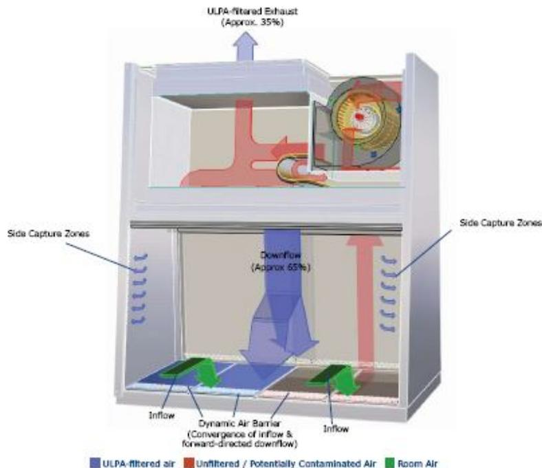
**Figure 1: Airflow Distribution Pattern in an LA2-4A1**
