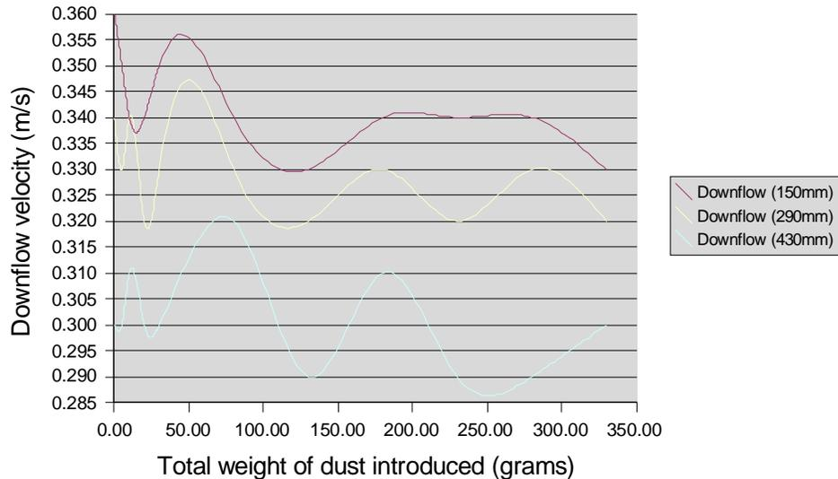
**Graph 3: Change in downflow at 2<sup>nd</sup> column of measurement points on NSF grid**
