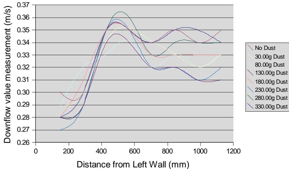
Graph 2: Change in downflow values at 1<sup>st</sup> row of measurement points on NSF grid
