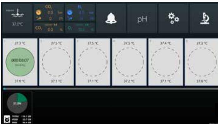
The main screen shows all 6 chambers as each counter illustrates the duration of time lapse recording done. At the upper right portion, snapshots of other useful information regarding the incubator such as temperature, pH measurement, CO<sub>2</sub> and O<sub>2</sub> status, and set points are displayed.
