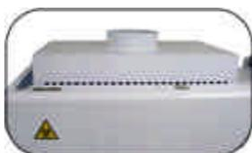
Thimble duct means that the collar has perforations to allow outside air to be pulled in as opposed to hard duct that has no holes. The exhaust collar is then connected to a duct tube connected to an external blower.
