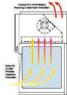
Class II BSC has inflow to protect the operator and a clean HEPA-filtered downflow to protect the product on the work tray as shown below. Because of dual protection offered Class II, is the widely used cabinet in the industry.
