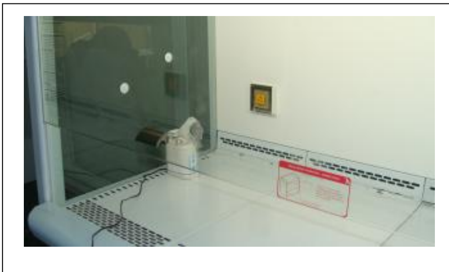
Figure 2. Smoke test to verify the air 'split' pattern
