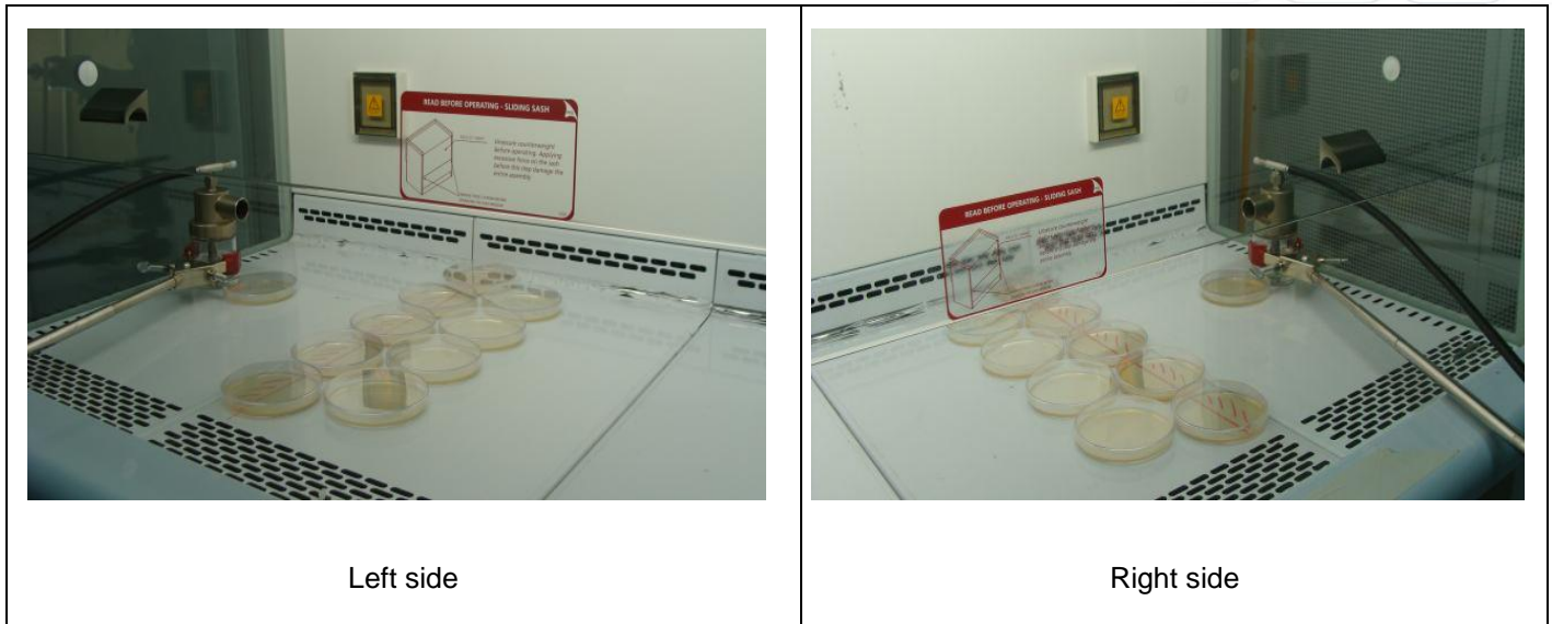
Figure 3. Cross contamination test with nebulizer placed at the actual air split point (1/3 work surface depth from back wall)
