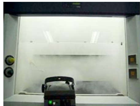
Figure 2. Gross visualization challenge at 0.3m/s. Smoke cleared within 6 secs and no smoke escaping from work chamber.
