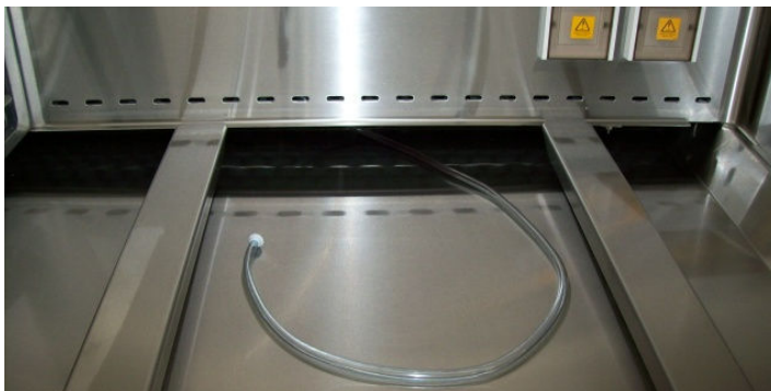
PAO sampling tube, located underneath the tray
