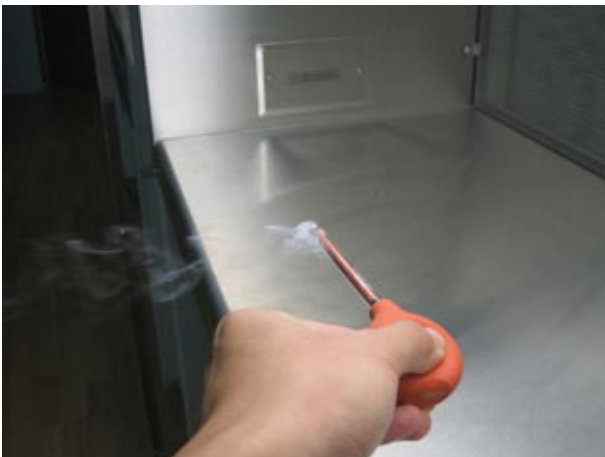
Figure 1: Smoke flowing out smoothly away from the cabinet away from object
