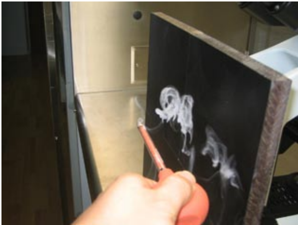
Figure 3: Vortices formed behind the microscope even with a board being placed.
