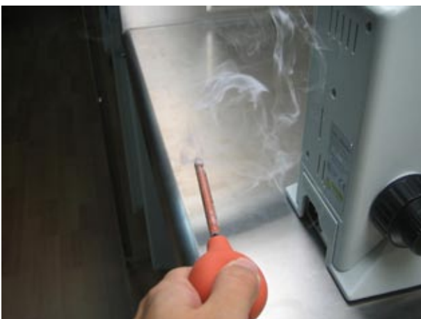
Figure 2: Serious vortices formed behind the microscope
