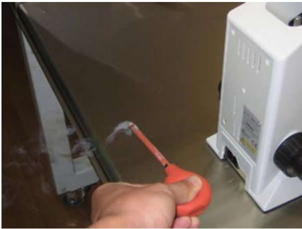
Figure 4: Smoke pattern in a vertical laminar flow cabinet
